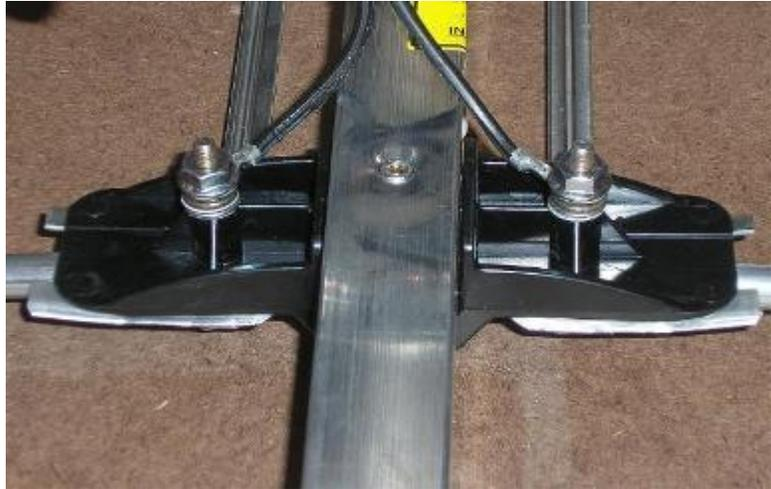
The routing of the twin lead wire should look like the picture on right.
