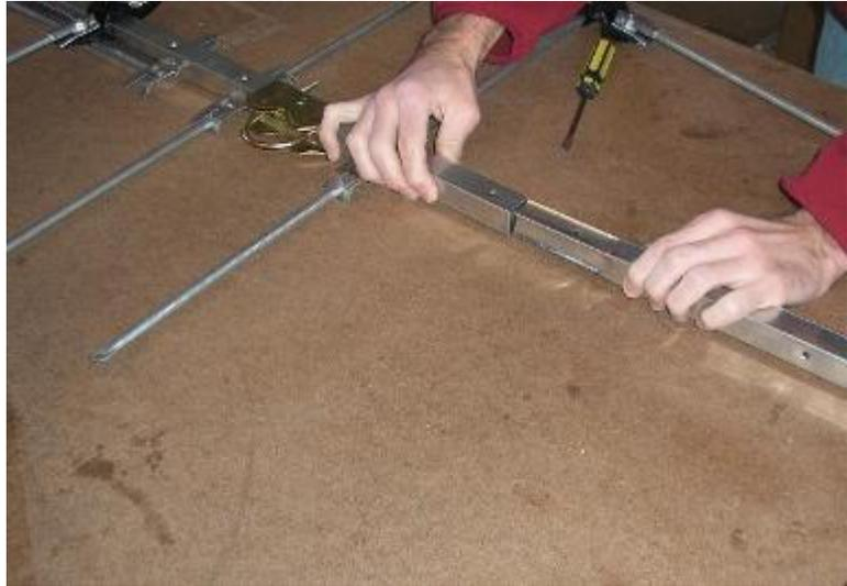
Place the element that was removed with the nut and bolt back onto the main boom and replace the nut and bolt as they originally were and tighten.
