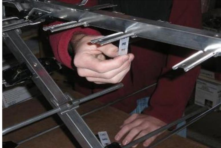
Line up the hole near the front of the UHF boom with the holes of the antenna brace. Insert a bolt and thread a small hex nut onto the bolt and tighten
