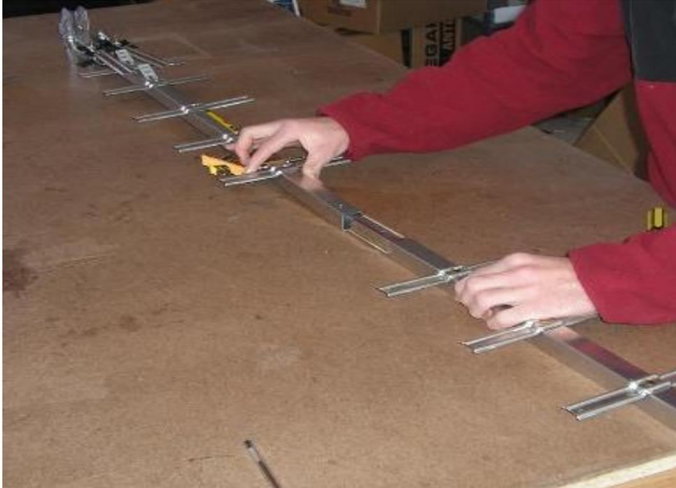
Slowly and carefully fold out the elements on both of the reflectors making sure they snap into place properly.
