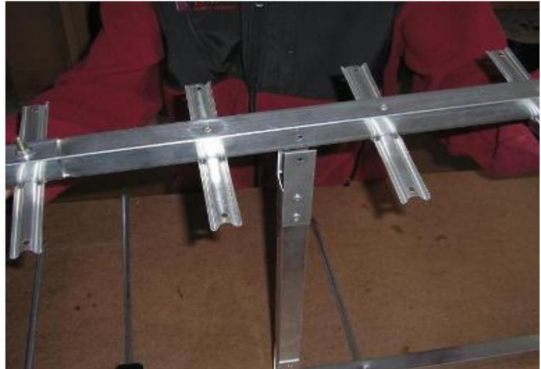
Slide the reflector into position between the struts located on the VHF boom. Line up the holes and insert a bolt. Thread a small hex nut onto the bolt and finger tighten.
