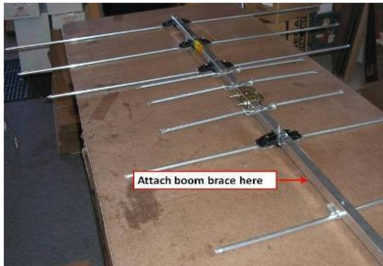
With the VHF antenna lying upside down slide either end of antenna boom brace over the VHF boom. Line up the holes of the brace and boom. Insert the bolt and thread one small hex nut onto the bolt and tighten
