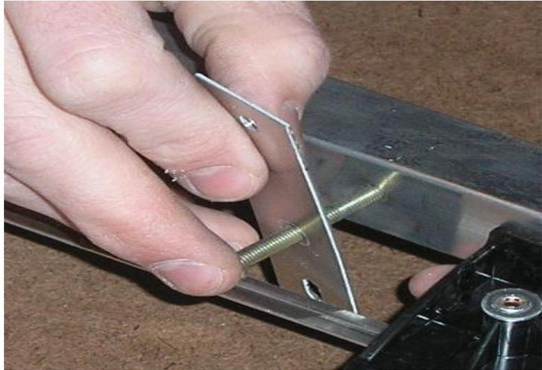
Connecting the VHF and UHF antennas together.
